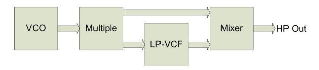
Then it's just a case of a little mixing, you'll find that the LP filtered signal is a little quieter than the direct signal, so set it to maximum and lower the volume of the direct signal until 100% phase cancellation occurs. In the above diagram you can use either the 12dB/Oct or the 24dB/Oct. So...... with this little filter you can do:
